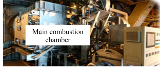
Fig.2. Grate firing system of the wood pellet.
